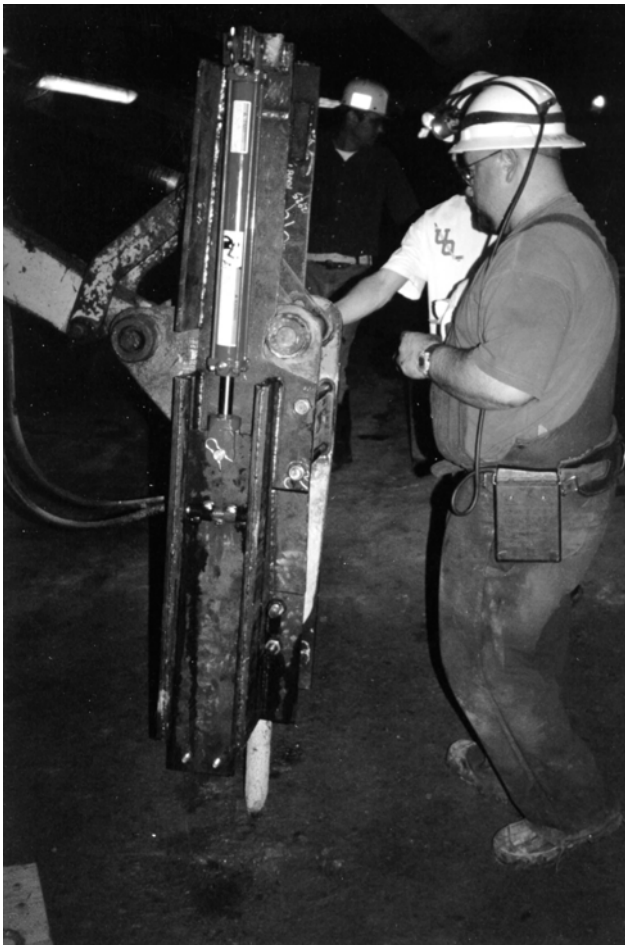
Figure 11.—Track-guided pincher arm attached to hydraulic impact hammer head.
