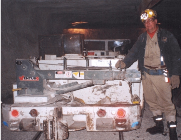
Figure 8.—Swing boom arm attached to mine vehicle.
