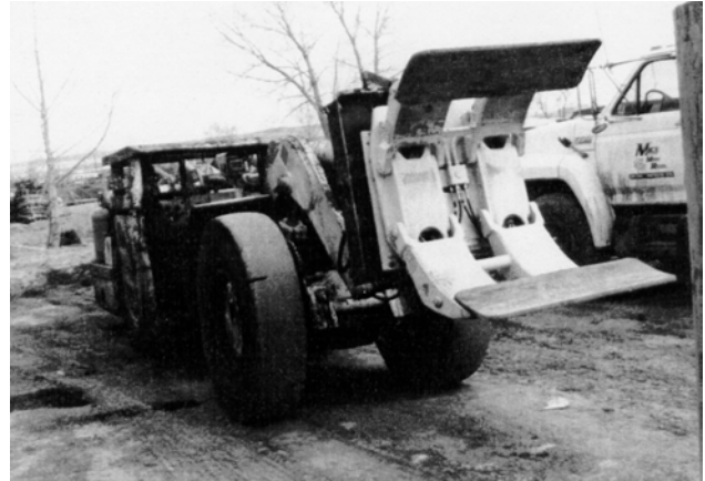
Figure 6.—Attachment used to pick up and maneuver can cribs.
