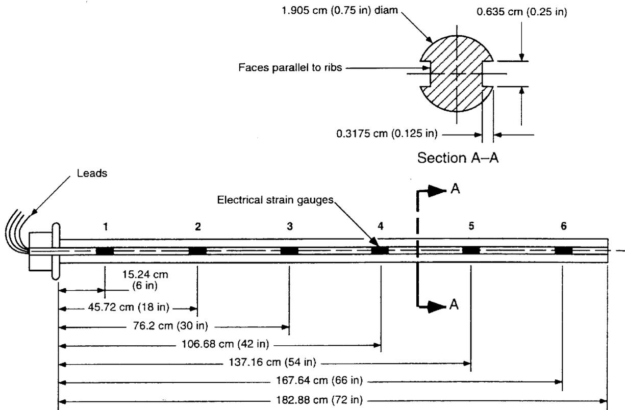
Figure 1.—Instrumented roof bolt
