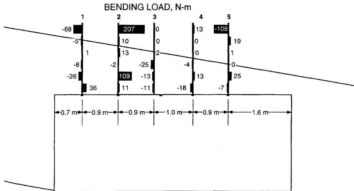
Figure 5.—Load profiles for test site 3
