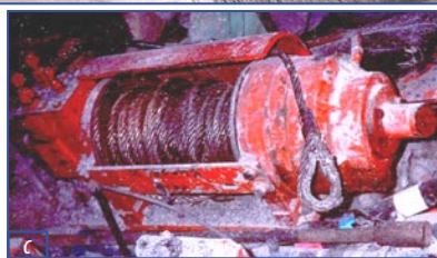
The screen tray of the MHS is tilted back toward the ground for the loading of a bundle of screen (a) by a remote-controlled winch (b,c).
