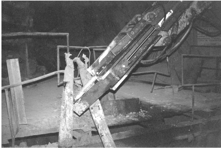
Figure 6.— Track-guided pincher arm picking up pipe debris from recessed grizzly
