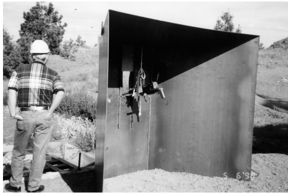
Figure 4.— Shield and industrial gun. (A) Setup for rock-breaking tests; (B) gun suspended from roof of shield.
