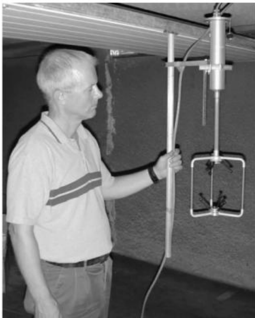
Figure 2. Three-axis ultrasonic anemometer
