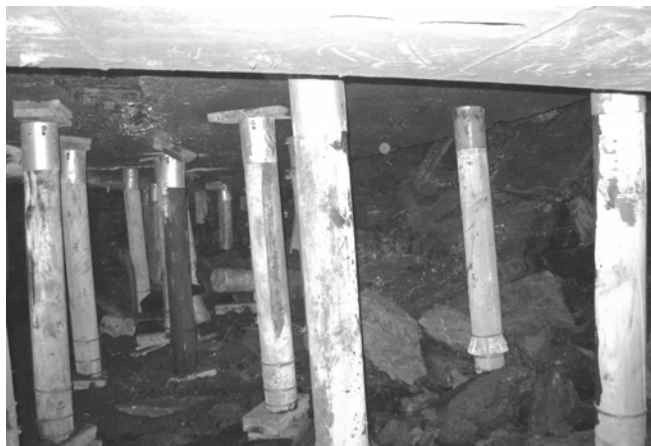
Figure 3. Engineered yieldable timber props equipped with active prestressing mechanical devices used as breaker line supports.
