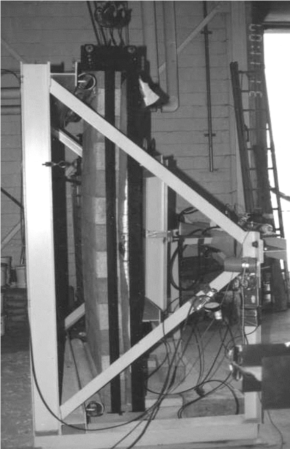
Figure 7. E-72 test fixture with test in progress, just prior to failure. The fixture has been modified to allow wedging to provide constraint at the top. The air bag that generates the lateral load is visible to the right of the test wall, near the center of the figure.
