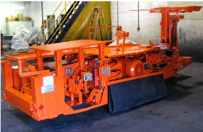
Figure 3. Roof bolter used for testing in underground coal mine.
