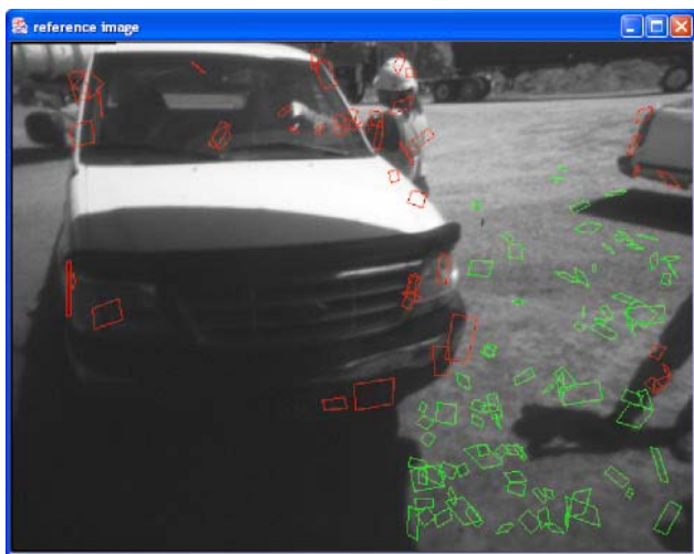
Figure 9. Captured image from one stereo camera with ground and alarm areas identified.
