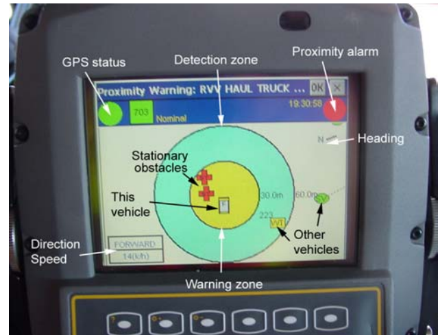
Figure 7. Driver interface for GPS-based proximity warning system.
