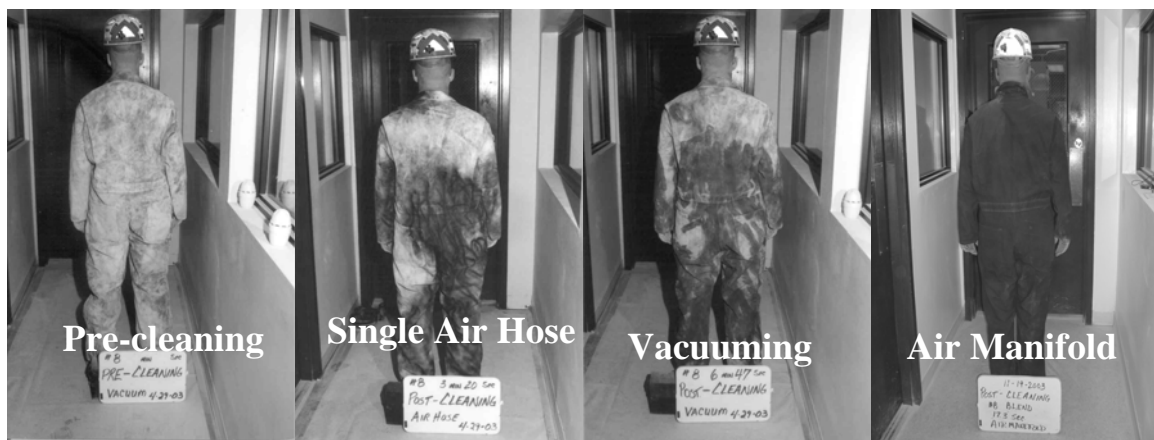
Figure 6. Effectiveness of various cleaning methods.
