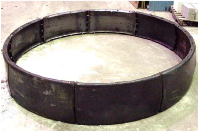
Figure 9. Single layer test of 9-ft diameter ring of tunnel liner plate (test conducted at NIOSH Mine Roof Simulator facility).
