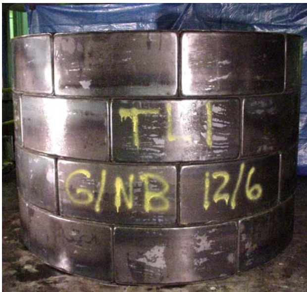
Figure 10. Full-scale test of four-ring assembly of tunnel liner plate in the Mine Roof Simulator.
