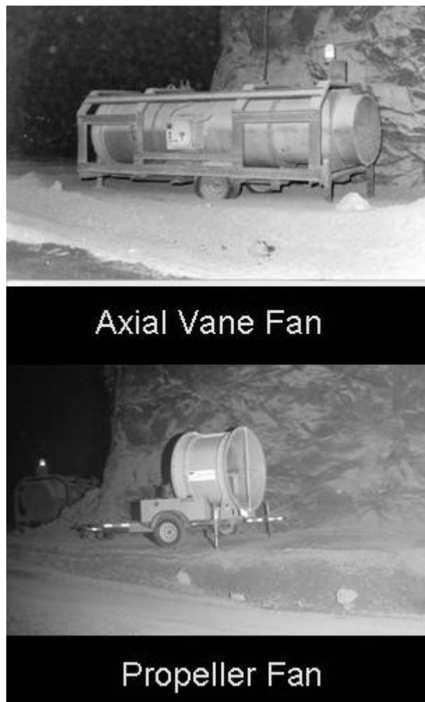
Figure 1. Axial vane fan and propeller fan used in study
