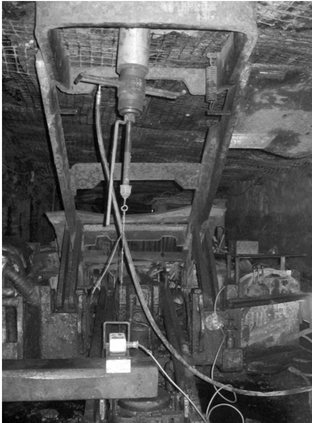
Figure 2. Pull test equipment showing reaction fixture, 20 ton hydraulic ram, 1-inch thread bar and string pot displacement sensor.
