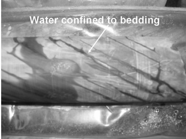
Figure 7. Water moves more readily along bedding than across bedding.
