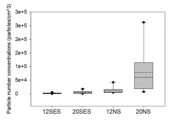
**Figure 1.** Particle number concentration (particles/cm<sup>3</sup>) in the breathing zone. Each box plot represents the 10th, 25th, 50th, 75th, and 90th percentiles. Solid circles indicate 5th (lower) and 95th (upper) percentiles. Dashed line defines mean.
