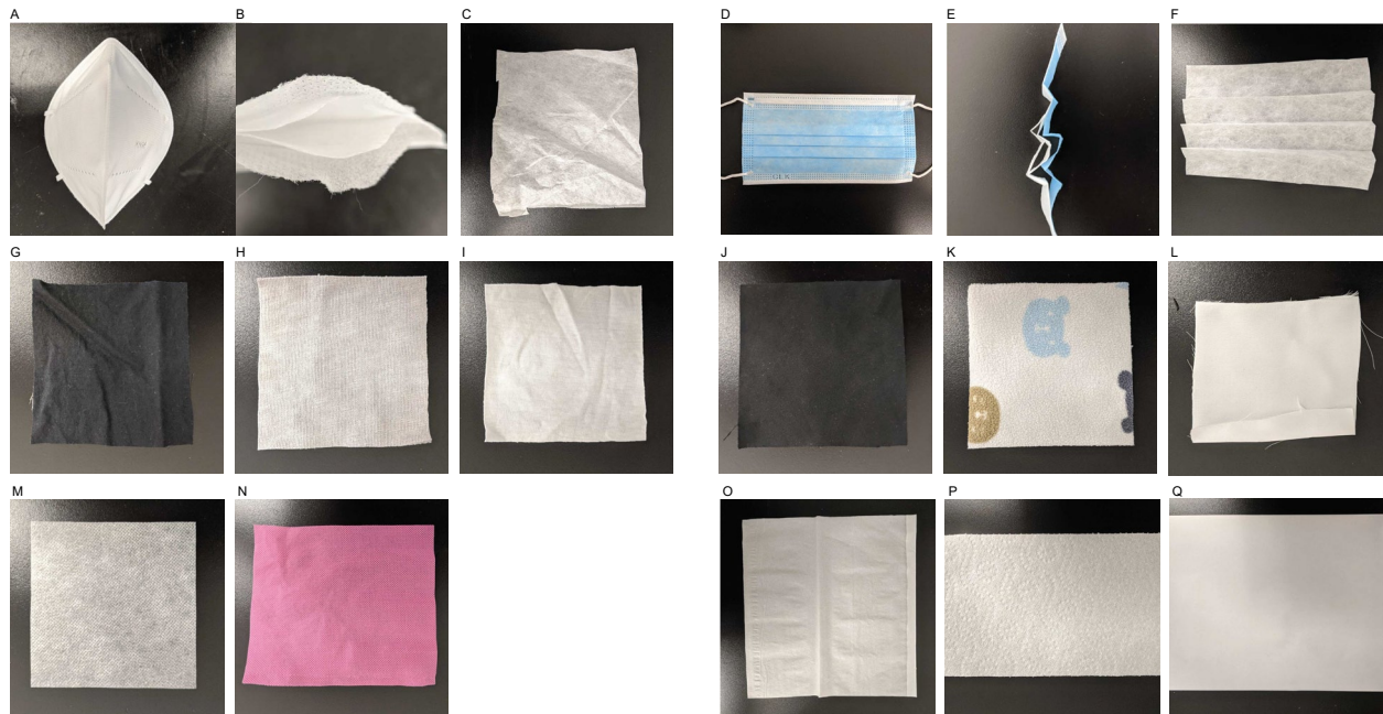
Figure S1. Optical images of reference and common materials. a-c. Reference material, 95% FFR. a. Image of a folded-style FFR. b. Cross section of said FFR showing layers of spunbond fabric (outer layers) and meltblown layers (inner layers). c. Meltblown fabric used in the actual experiments, it does not come from the FFR shown in a-b, due to limited amount of meltblown that can be used for testing from an FFR in a whole sheet. d-f. Reference material, medical face mask. d. Image of the surgical flat mask. e. Cross section of the medical face mask showing spunbond, meltblown, spunbond structure. f. Meltblown extracted from the mask used in main text Table 1, to be comparable with the 95% meltblown. g-i. Common materials, cotton 1-3 (respectively). A variety of cotton with different thickness and structure were selected, the data is given in Table 1. j-l. Common materials, nylon, polyester, and silk, respectively. m-n. Common materials, polypropylene spunbond 30 (PP-4) and 70 g/m 2 (respectively). o-q. Common paper-based cellulose materials, tissue paper, paper towel, copy/printing paper, respectively.
