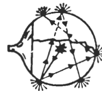
Figure 5.—Use of surface patterns to control light distribution.
