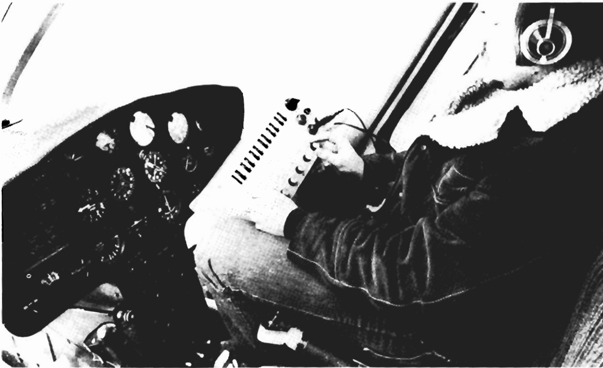
FIGURE 10. - Operation of the helicopter ULF EM receiver during field trials.
