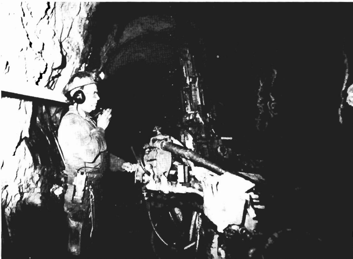
FIGURE 21. - Fan-hole drill operator wearing portable radio and special accessories in metal mine.
