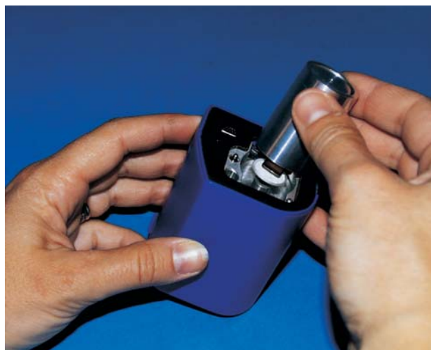
Figure 3-Installing a sample filter in the mass sensor.
