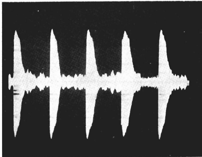
Figure 4-13. Received Surface Signals from 2500 Hz Transmitter, 1150 feet Underground
