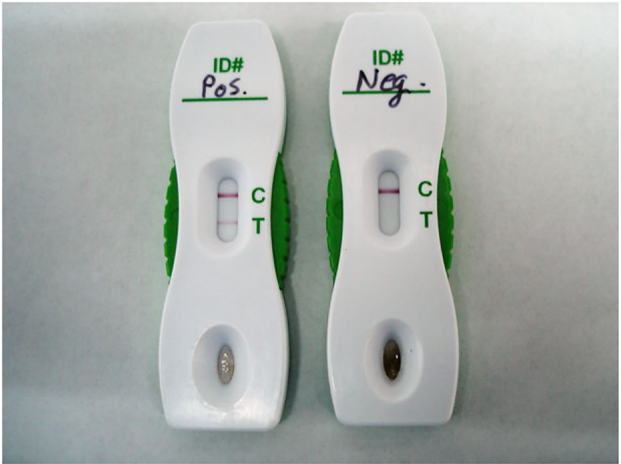
Figure 1. The Anthrax Active Detect Lateral Flow Immunoassay cartridges, showing positive (left) and negative (right) reactions. ‘T’ is the Test line and ‘C’ is the Control line.
