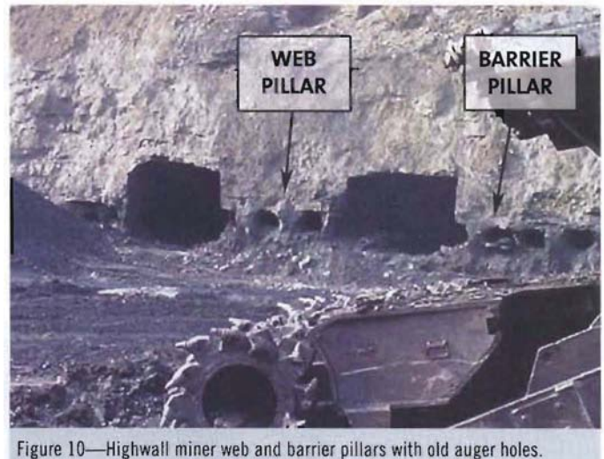
Figure 10—Highwall miner web and barrier pillars with old auger holes.
