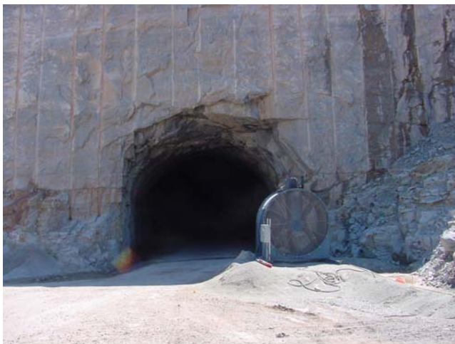
Figure 17. Site one, 2.44 m (8 ft) propeller fan blowing into a dual-entry large-opening mine.
