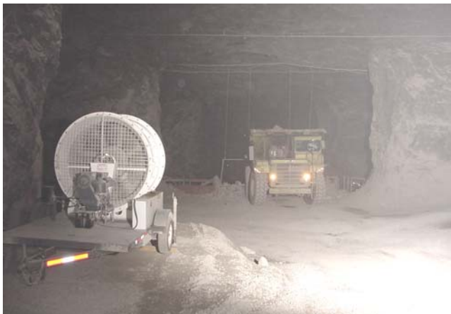
Figure 12. 1.37 m (54 in) diesel powered propeller fan used for face and regional mine ventilation.
