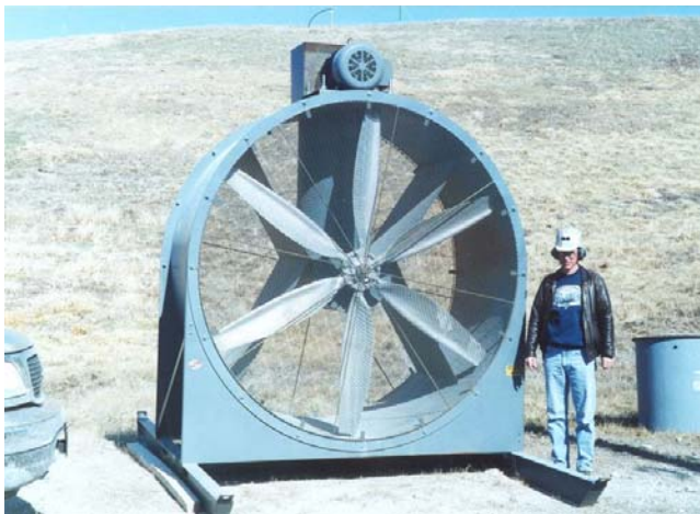
Figure 5. 2.4 m (8 ft) propeller fan used in study.
