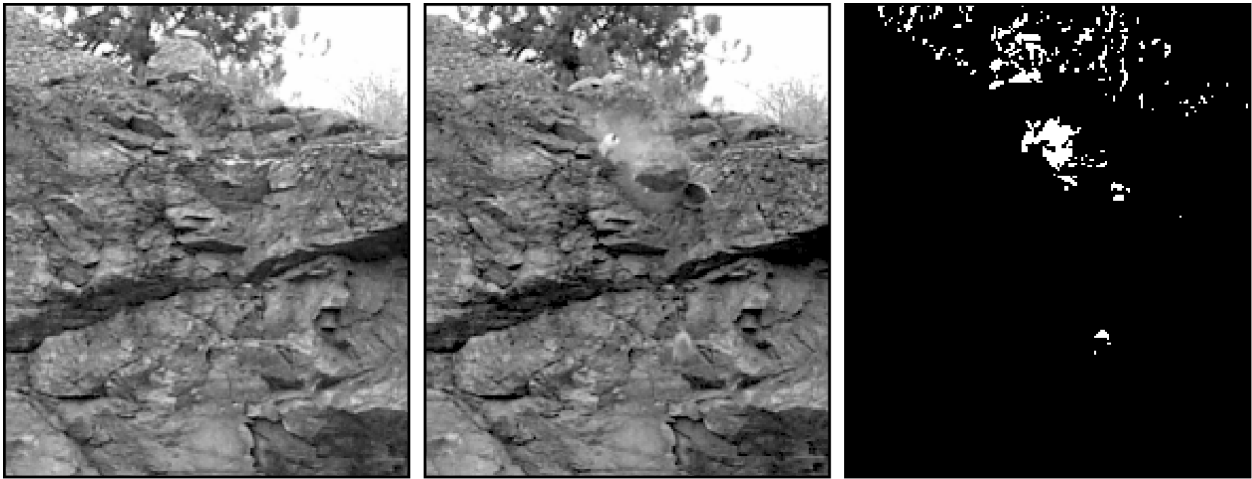
Figure 8. —In a rockfall experiment, rocks positioned at the top of a highwall are shown in the left image, the rocks falling are shown in the middle image, and the difference image with a threshold adjusted to enhance changes is shown on the right.
