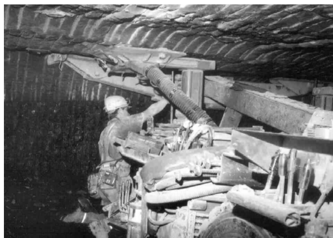
Figure 4. Canopy air curtain installed on roof bolter.
