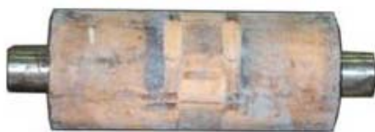
Figure 10. Coated tail roller for the CM.
