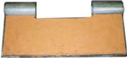
Figure 14. Coated slide plate for the continuous miner.
