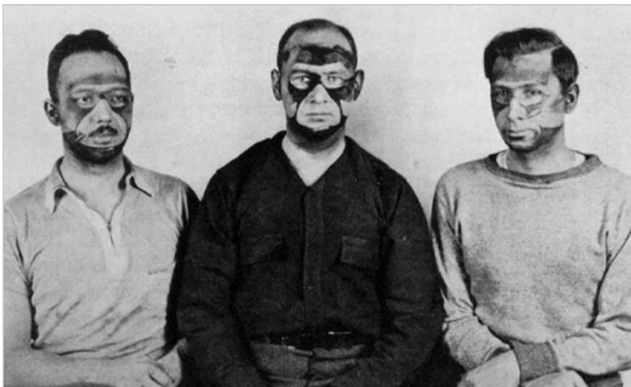
Figure 1. The effects of face seal leakage by intentionally producing mask leaks by inserting toothpicks under the facepiece. 4
