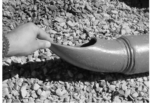
Figure 3. Directional elbow for bulk fill placement.
