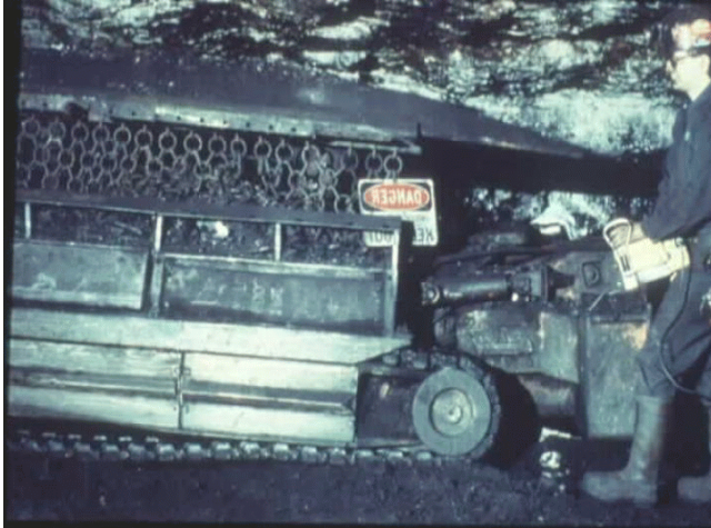
Figure 8. A Mobile Roof Support (MRS).
