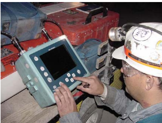
Figure 1: Engineer using the SIR-2 unit.
