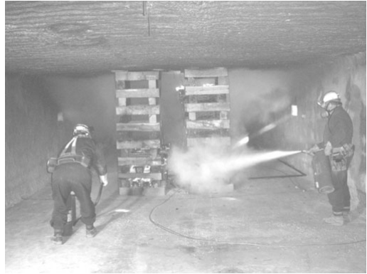
Figure 6. Use of fire extinguishers during crib block fire test No. 5.
