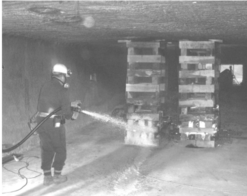
Figure 5. Use of gas-enhanced foam during crib block fire test No. 4.
