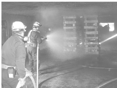
Figure 4. Use of fire hose during crib block fire test No. 3.
