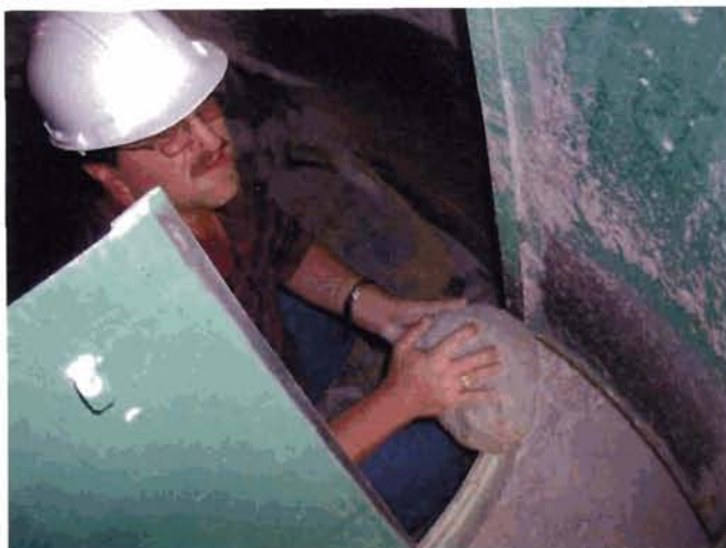
Figure 4b. Worker easily removing large rocks when using door.
