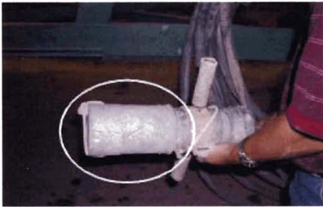
Figure 2. The rubber “boot” to protect the male cable connector from dirt, dust, and damage.
