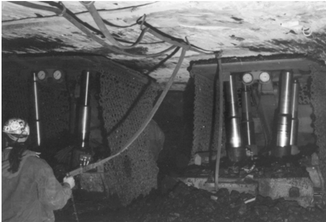
Figure 4. Full pillar extraction using mobile roof supports.
