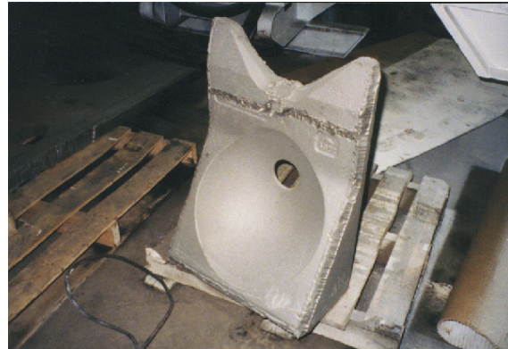
Fig. 14 “Zipper-shaped” leg cylinder casting to avoid stress concentration caused by orientation of casting to principal stress field
