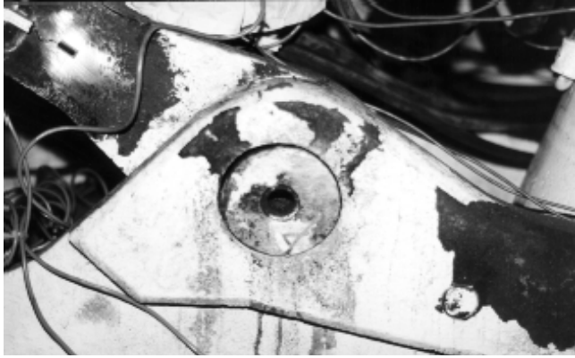
Figure 6 Reduction in lemniscate pin contact area for worn joint
