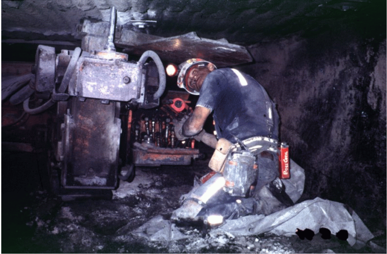
Figure 1. Roof bolting in a low seam mine often requires workers to maintain awkward postures.
