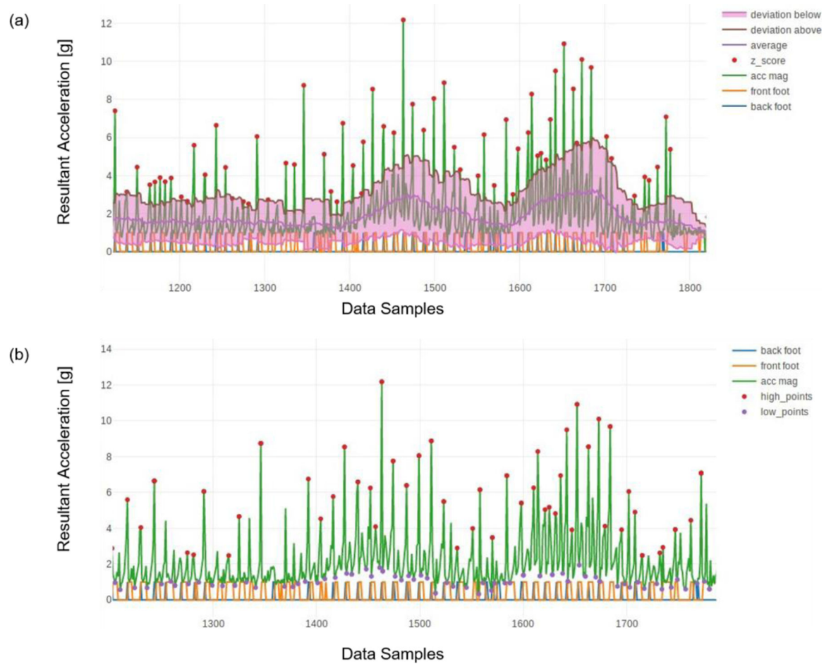
Figure 8. (a) Z-Scoring for peak detection (b) Peak Detection Gait event (heel contact and toe off) identification from accelerometer scalar magnitude (or resultant acceleration) and the pressure FSRs
