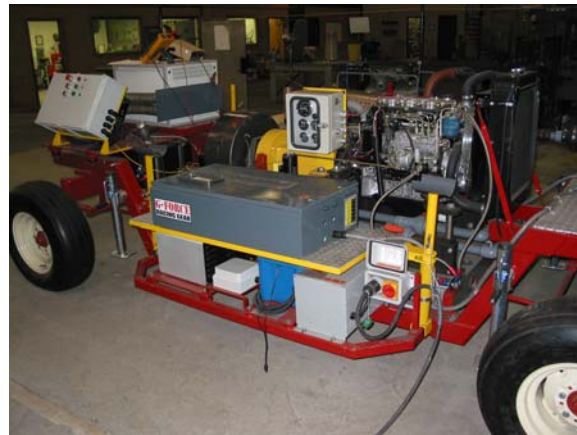
Figure 3. 150 kW dynamometer/Isuzu C240 system
