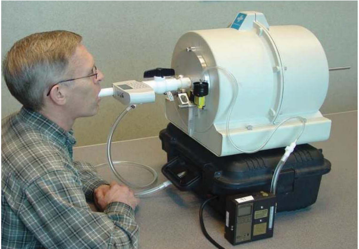
Figure 4. Cough aerosol sampling system for collection of influenza aerosols. (Courtesy of William Lindsley.) With this system, the patient or research participant breathes and coughs into a mouthpiece connected to a spirometer. The aerosol particles expelled by the patient are then collected by an aerosol sampler (yellow and black) attached to the spirometer. The brown instrument on the outside is a vacuum pump that pulls air through the aerosol sampler.
