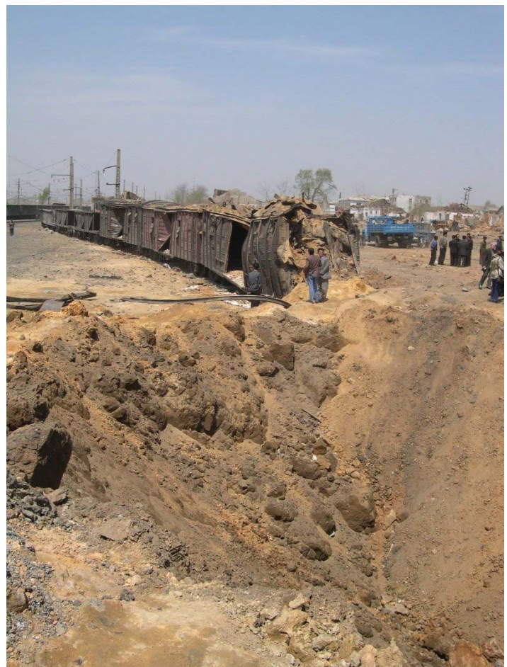
Figure 2. Crater produced by train explosion in Ryongchon, North Korea. Accident may have been the result of cars of AN coming into contact with electrical wires.”
