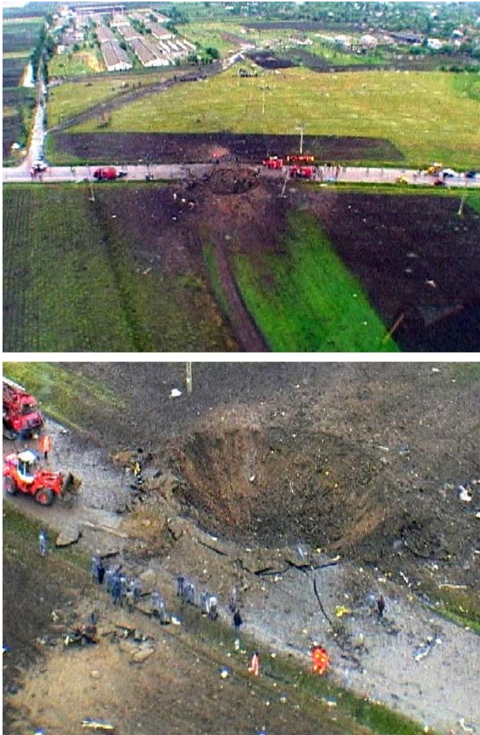
Figure 4. Accident in Romania in which 20 MT (22 t) of "nitrous fertilizer" caught fire and exploded, killing 17 people.
