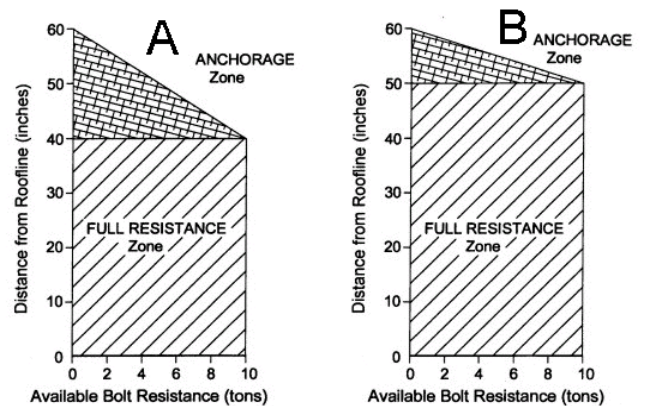
Figure 5. Effect of the Grip Factor on the resistance available from 10-ton roof bolts to react against roof loads. (A) Grip Factor = 0.5 tons/in; (B) Grip Factor = 1.0 ton/in.
