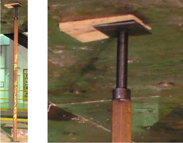
Figure 6. Wedged prop for eccentric loading.
