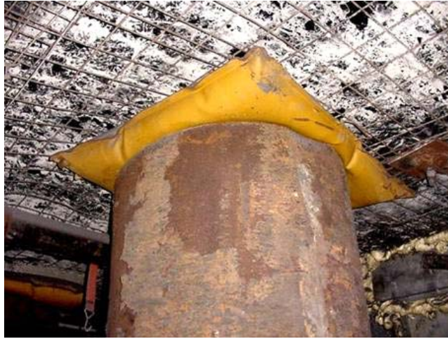
Figure 3. Prestressing Unit used in conjunction with Can Support.
