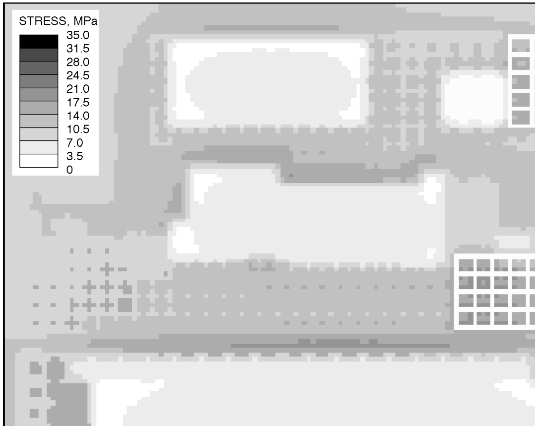
Figure 6. Vertical stress distribution for lower seam 2, step 2.
