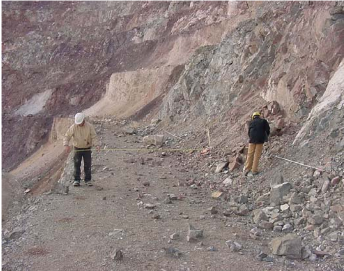
Figure 2: Students measuring the bench width and idealized cross section.
