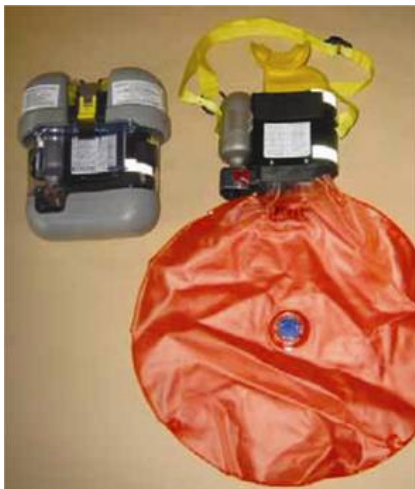
Figure 7. Partially Uncased and Uncased Ocenco M-20 Self-rescuer
