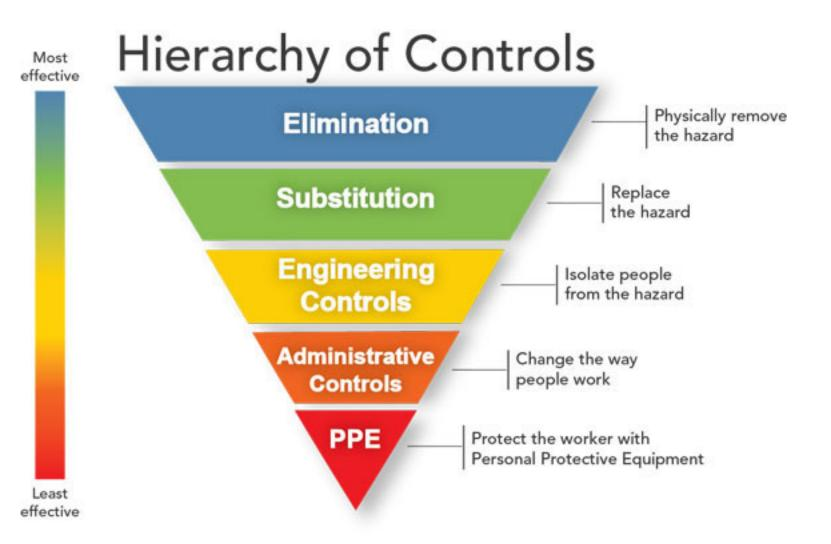
Controlling exposures to occupational hazards is a fundamental way to protect personnel. Traditionally, a hierarchy controls approach has been used to achieve feasible and effective control. Some of the control measures may fall integrated that multiple categories. It should also be emphasized that multiple control strategies can be implemented concurrently a or sequentially. This hierarchy can be represented as follows:
