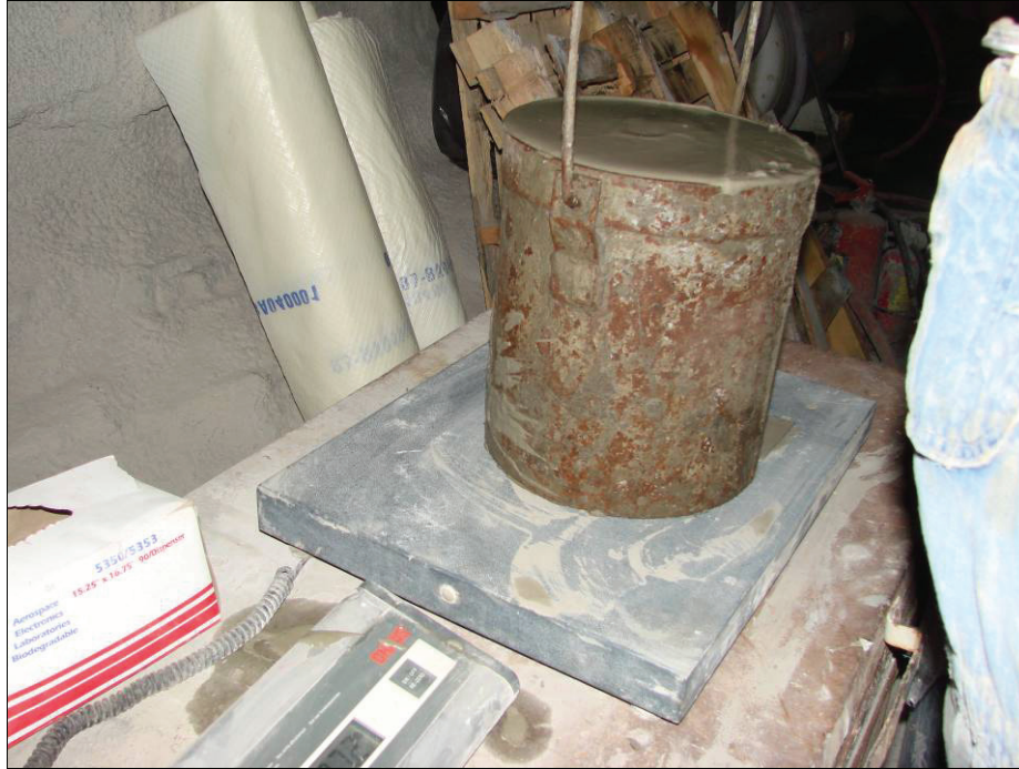
Figure 10.—Digital scale and bucket used to calculate the density of the cementitious foam slurry.
