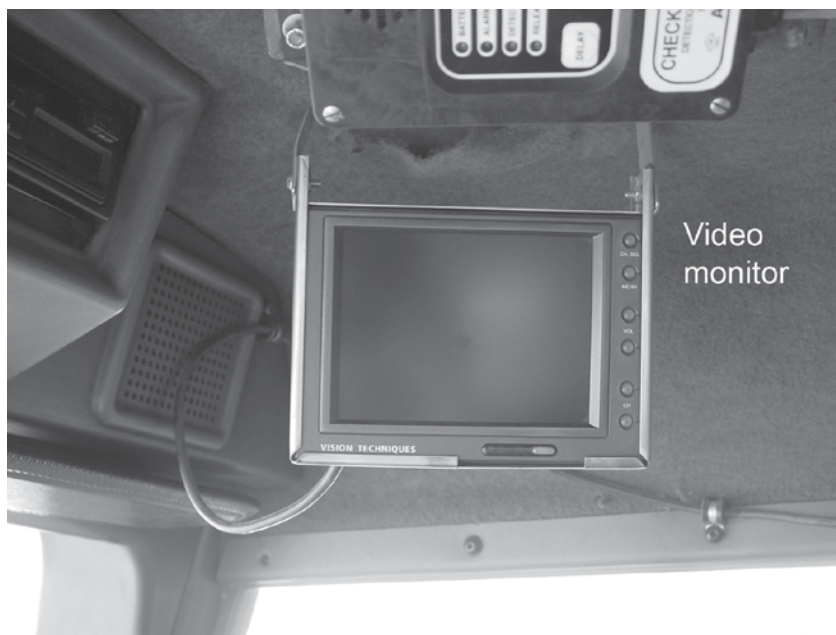
Figure 28. Example of LCD video monitor mounted in the upper right corner of truck cab.
