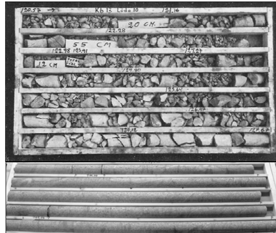
Figure 1.—The contrast shown by these two core boxes suggests orders of magnitude differences in quality. Quantitative descriptions of shear strength and deformation modulus would vary by orders of magnitude as well. Quality descriptors like RMR or GSI that suggest qualities differing from only 5 to 95, or 10 to 90, cannot then be as appropriate as the 0.001–1000 range of Q seen in these examples. Increasing the range of Q to Q_c adds further reality, since Q_c might range from 0.0005 to 2500 in these two cases.
