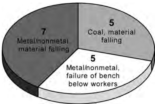
Figure 3. Pie chart showing numbers of fatalities in coal and metal/nonmetal surface mines caused by failure of benches above and below workers for the period 1996-2000. Failure of benches above allows material to reach workers. Failure of benches below causes workers, especially those operating heavy equipment, to fall with falling bench material.
